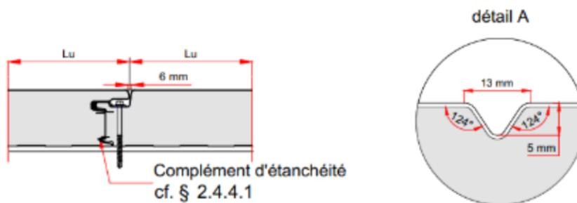
Figure 2 – Panneau sandwich isolant Evolution Multi Groove
