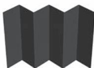
Angle rentrant bardage horizontal
